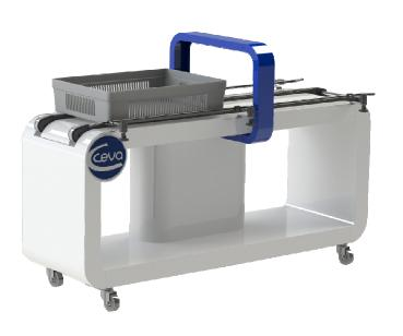
Our new **Desvac Gel Dispenser** is a unique equipment capable of evenly dropping vaccine in a gel form on Day Old Chicks. The Coccidiosis vaccine is absorbed when the birds ingest the red coloured droplets. Our equipment is designed to dispense the vaccine uniformly on the crate ensuring best possible cover, contributing to good vaccine take.
